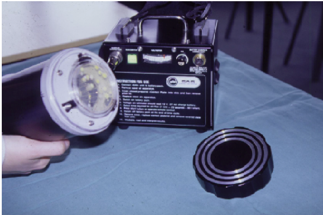
Figure 1. Surface Air Sampler (Cherwell Laboratories, Bicester, UK).
